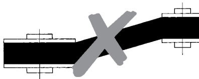
Axial misalignment of sheaves
